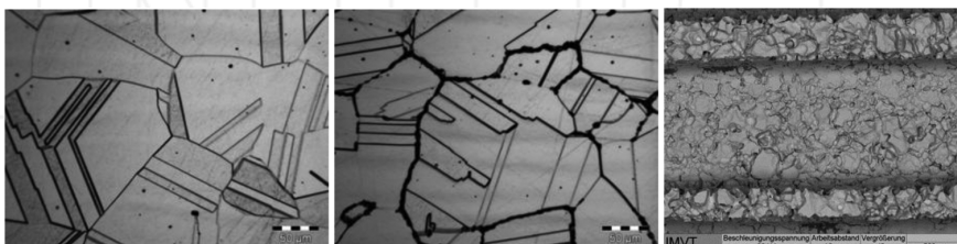
Figure 12. Micro-structure of Hastelloy C-22 (2.4602). Left: after quenching from 1100°C/70 min in water. Middle: after cooling from 1100°C with a rate of 3 K/min (1100°C ≥ 650°C = 2.5 h). Right: corrosion attack after diffusion welding in 95–97% sulphuric acid at 100°C and 1008 h.
