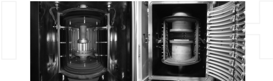
Figure 22. Diffusion bonding furnaces. Left: Maytec diffusion bonding furnace, maximum force 20 kN. Right: Systec diffusion bonding furnace, maximum force: 2 MN.
