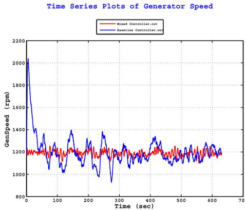
Figure 8. Generator speed
