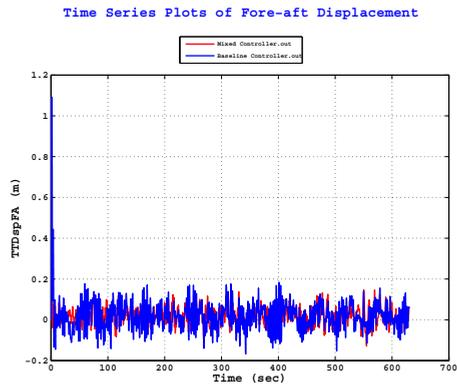
Figure 9. Tower fore-aft displacement
