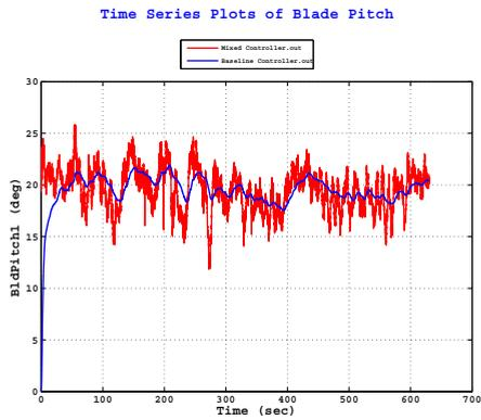
Figure 10. Blade pitch angle
