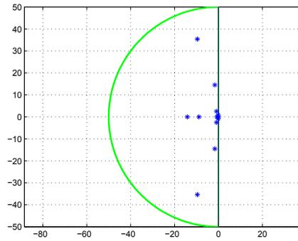
**Figure 5.** Closed loop poles
