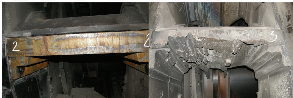
Figure 2. New grinding table (left) and worn grinding table (right).
