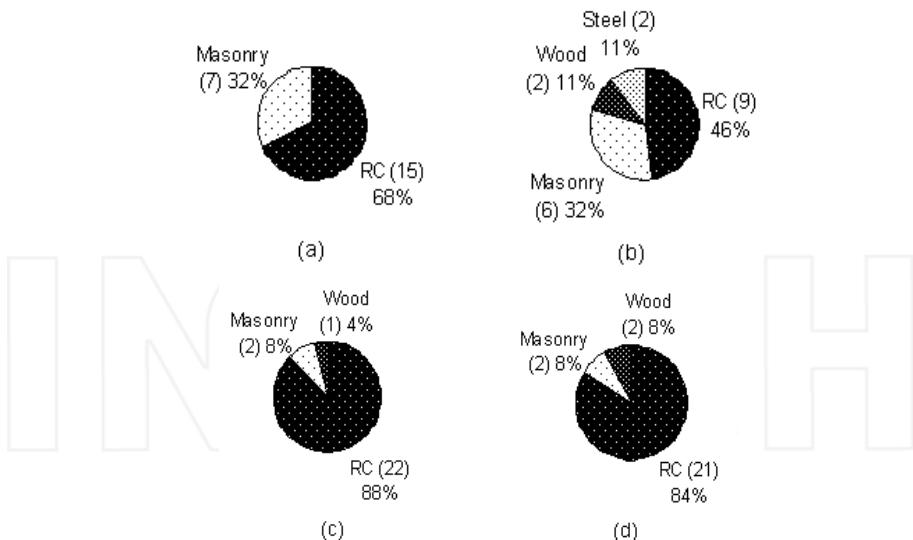
**Figure 5.** Type of construction for (a) mosques, (b) minarets in Bolu; and (c) mosques, and (d) minarets in Duzce and Kaynasli (number of mosques/minarets is given in parenthesis)
