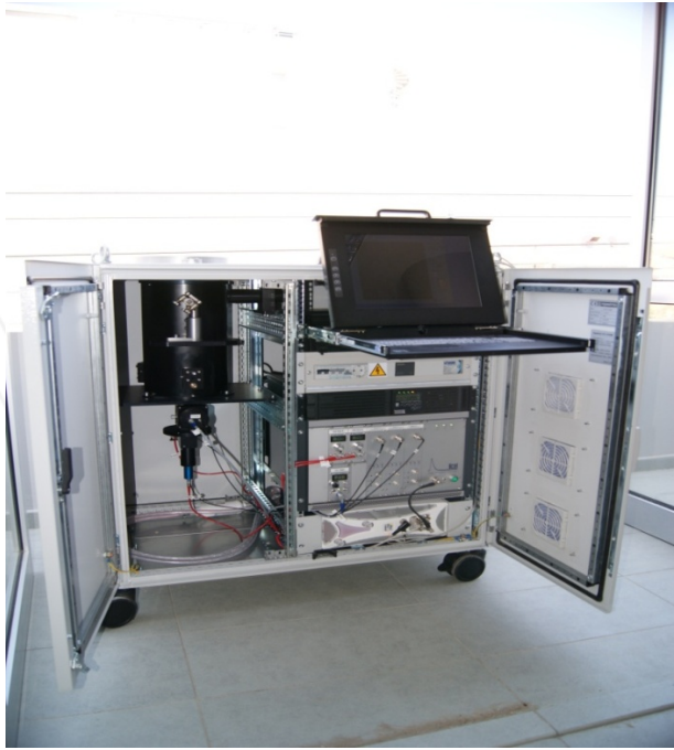
Figure 3. CUT's Depolarization Lidar System
