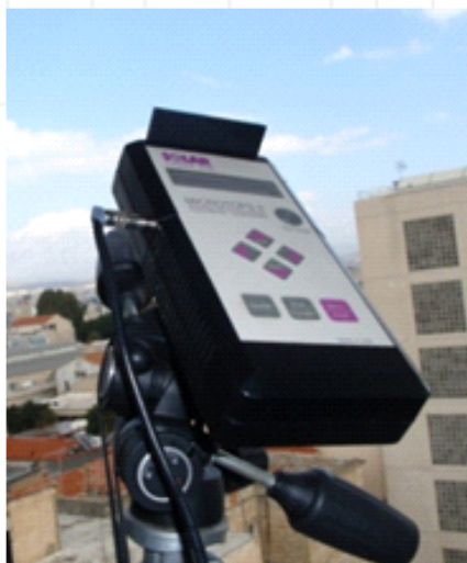
Figure 2. MICROTOPS II handheld sunphotometer
