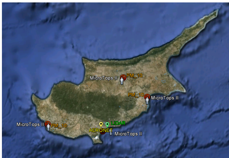
Figure 8. Overview of the available instrumentations at the selected sites within AIRSPACE project. Limassol was the main site (LIDAR, AERONET, PM), Nicosia validation site (MicrotopsII, PM); 15-day campaigns were conducted at Larnaca and Paphos.
