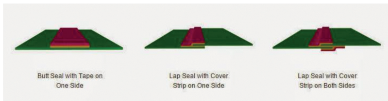
Figure 2. Schematic presentation of a hot air/wedge welded seams [12].
