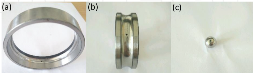
Figure 19. Simulated bearing faults: (a) outer race fault; (b) inner race fault; and (c) ball fault.
