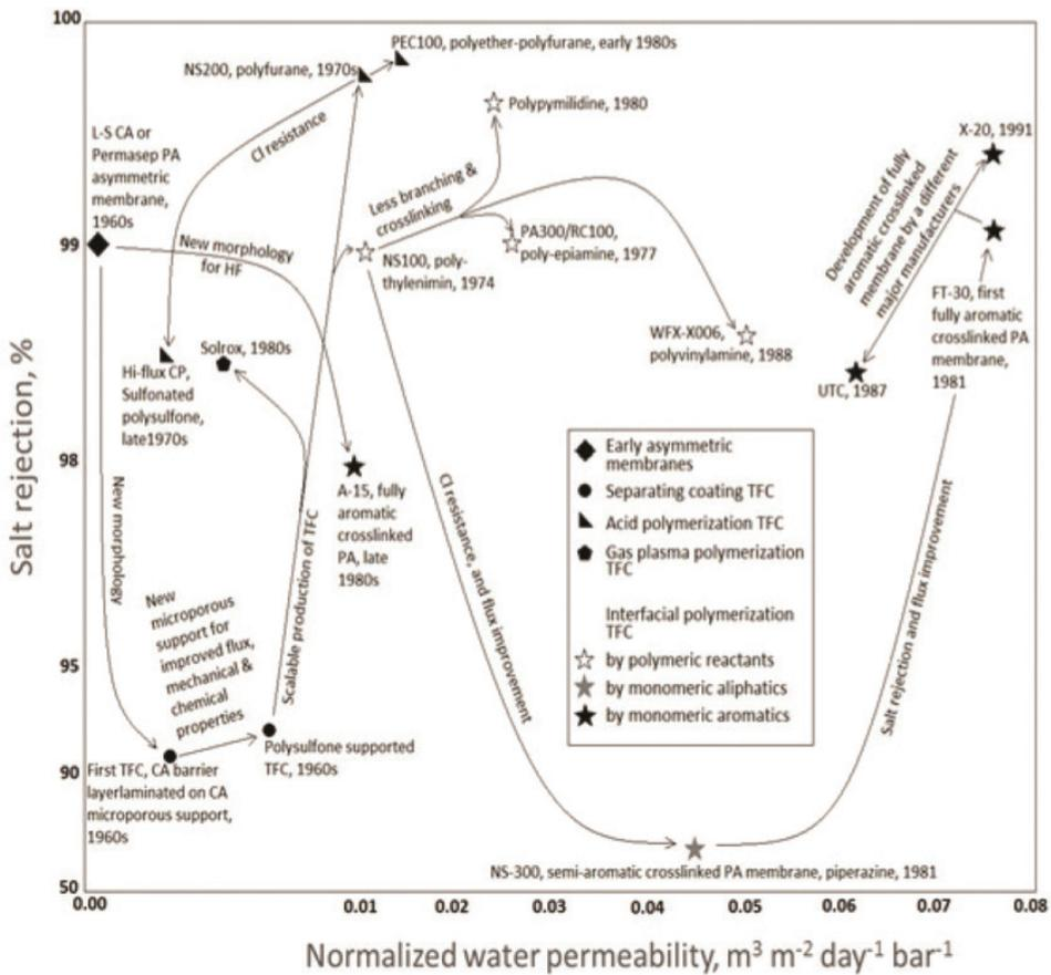
Figure 2. Development of thin-film composite RO membrane [30].
