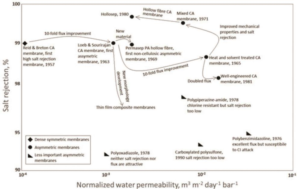
Figure 1. The development of asymmetric RO membranes [1].
