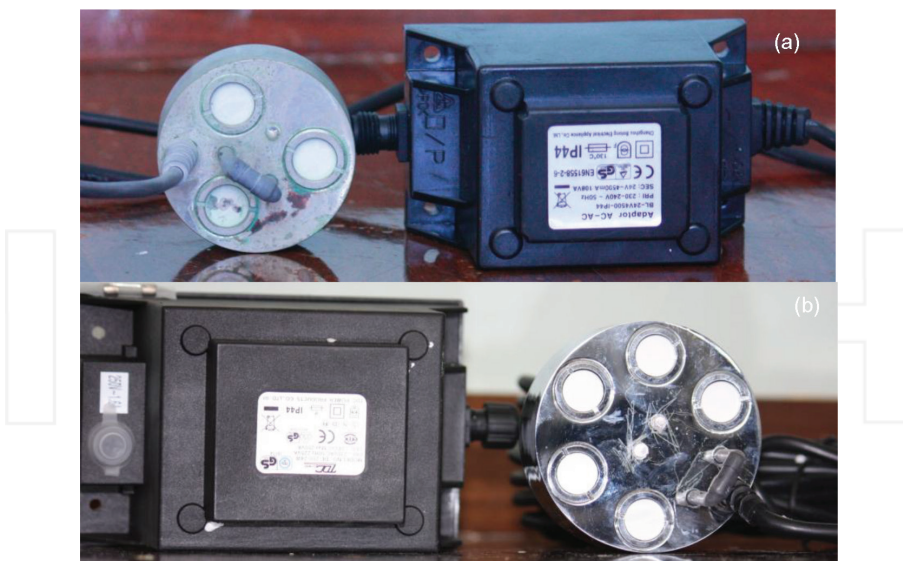
Figure 7. Ultrasonic nebulizers employed in the study: (a) shows the 1.7 MHz ultrasonic nebulizer with power supply unit and (b) shows the 4.8 MHz ultrasonic nebulizer with power supply unit.
