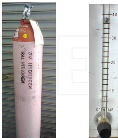
Figure 7. Bottled syngas (left) and fuel flow rotameter (right).
