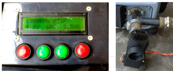
Figure 6. Digital display (left) and air servo valve (right).
