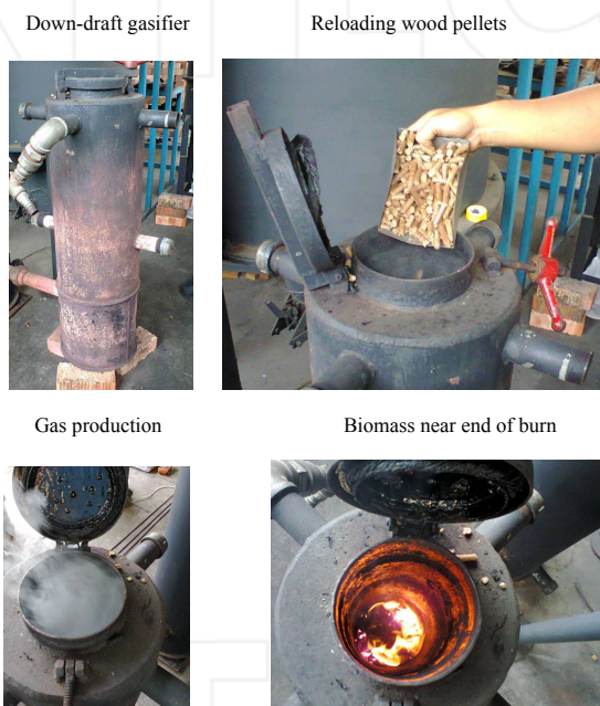
Figure 8. USM's 5 kW down-draft wood pellet gasifier.
