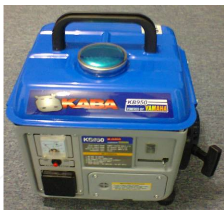
Figure 2. The Yamaha 950, 650 W genset, assembled by Kaba.
