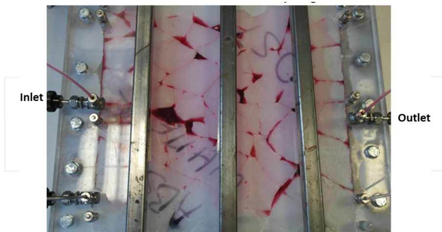
Figure 6. A square marble tile was fractured and reassembled within an aluminium frame sandwiched between two Plexiglas plates. The fracture network consisted mainly of narrow fractures with 12 large fractures. The vulgar open fractures were larger bodies of open space varying between 0.4 and 2.2 cm aperture. These cavities were used to observe the advancing foam front during co-injection. In this figure, the marble tile model is filled with red-dyed brine to emphasize the fracture network.
