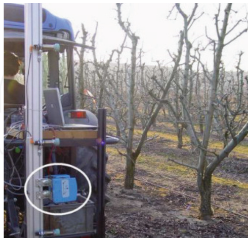
Figure 14. LIDAR placed on the back of a tractor [28].
