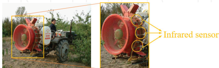
Figure 1. Photo of the automatic target-detecting orchard sprayer working in orchard [6].
