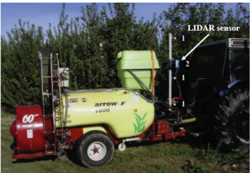
Figure 13. Variable-rate orchard sprayer prototype implemented with LIDAR sensor [13].
