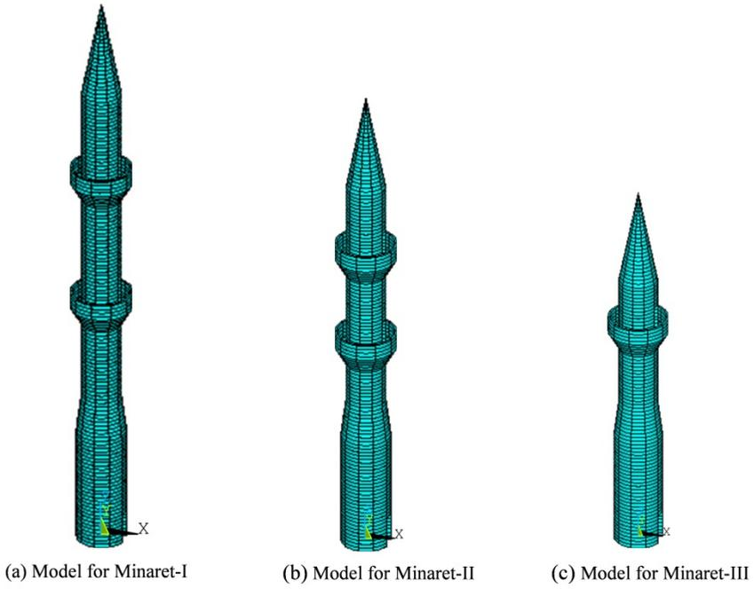
**Figure 12.** Finite element models of the three minarets
