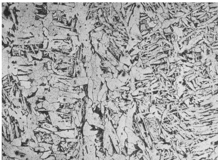
Figure 25. Weld, Nital Etch, magnification 250 \times , ferritic-pearlitic dendritic structure.
